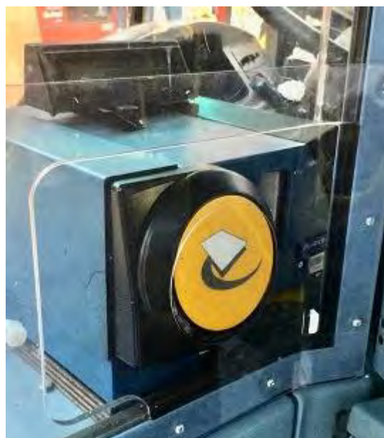
Figure 6_2: Flexible plastic over the top of Smart Card Reader pad. Held in place by a removable polycarbonate panel
