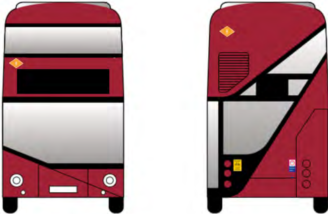
Figure 10_4 Front (left) and Rear (right) Propulsion Identification Symbol location
